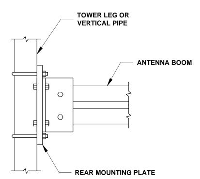
FIGURE 1 REAR MOUNTING PLATE
