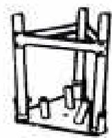
GNBP Base Plate with DMBS Base Stubs driven into the ground through 3 holes
